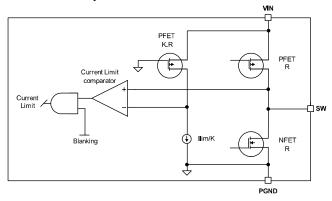
Figure 4. Current Limit Detail
