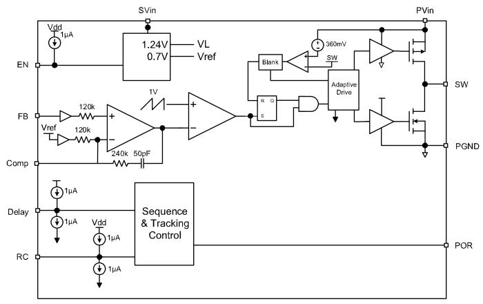
Figure 1. MIC22400 Block Diagram
