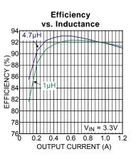
Figure 3. Efficiency vs. Inductance
