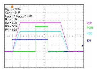
An alternative method here shows an example of a V<sub>DDQ</sub> & V<sub>TT</sub> solution for a DDR memory power supply. Note that POR is taken from Vo1 as POR<sub>2</sub> will not go high. This is because POR is set high when FB >  $0.9 \cdot V_{REF}$ . In this example, FB<sub>2</sub> is regulated to  $\frac{1}{2} \cdot V_{REF}$ .
